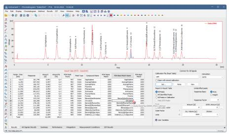
Fig. 18: Chromatogram with PDA - Results Table
