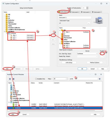
Fig. 3: System Configuration
