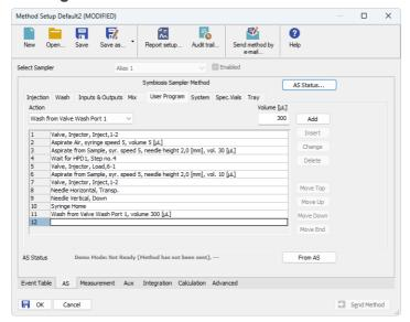
Fig. 10: Method Setup - AS - User Program
