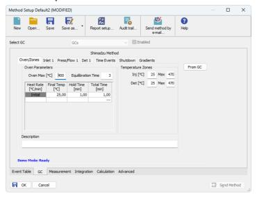
Fig. 6: Method Setup - GC - Oven/Zones
