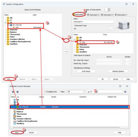
Fig. 4: System Configuration
