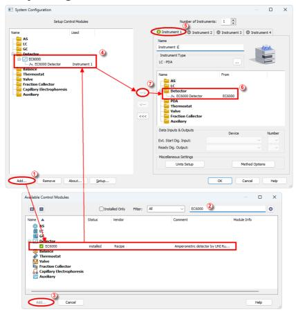
Fig. 3: How to Add Recipe EC6000 module
