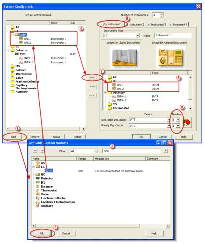
Fig 2: How to add Flom 301M pump
