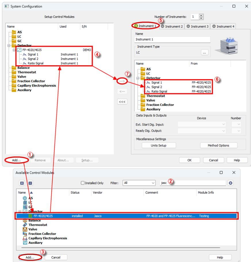
Fig. 3: How to Add Jasco FP-4020/4025 module
