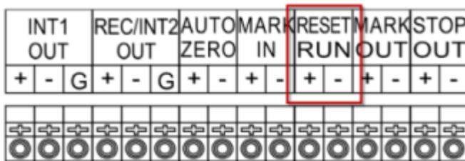
Fig. 2: Jasco FP-4020/4025 rear panel: Input/Output Terminals
