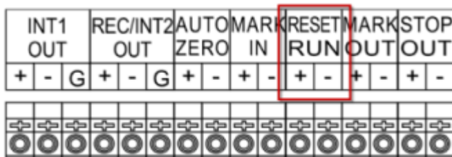
Fig 2: Jasco FP-4020/4025 rear panel: Input/Output Terminals
