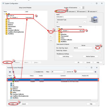
Fig. 3: How to Add Kontron 460/465 module
