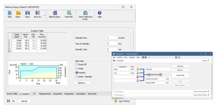
The setting of the instrument method as well as online monitoring, is seamlessly integrated within Clarity
